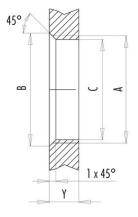
Installation direction: o-ring sits on chamfer.
